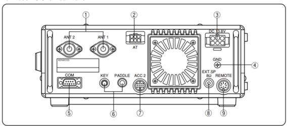
Attach an Antenna or Two Antennas.
